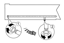
After installation, use soapy water to check connections for leaks.
