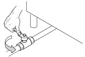
Clean the pipes to remove any dust, dirt or foreign matter which could block the supply.
